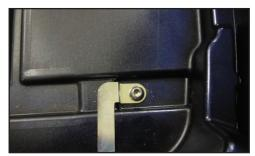
Connect the black wire with white marking tape from the CB antenna cable to the lower threaded hole in the antenna base with the provided Philips head screw.
